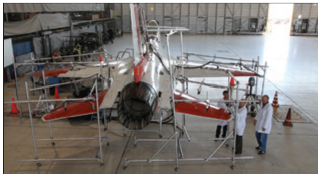
Figure 1. Ground vibration test (GVT) on an aircraft at Edwards Air Force Base.
