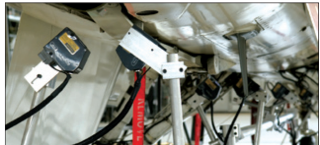
Figure 8. Biaxial DOFs on aircraft belly.
