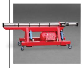
Moog Engineering provides shock testing services with a test system that is ideally suited for quick turnaround while minimizing over-testing. The system uses high energy mechanical impacts to replicate pyrotechnic events. Typical test articles are flight hardware and avionics. SRS levels can usually be replicated within a short lead time, and levels in excess of 40,000 Gs are generally easy to obtain on test articles weighing less than
