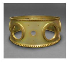
ESPA mounts to the standard NSSL (formerly EELV) interface bolt pattern (Atlas V, Falcon 9, Delta IV, OmegA, Vulcan, New Glenn) and is a drop-in component in the launch stack. Small payloads mount to ESPA ports featuring either a Ø15-inch bolt circle with 24 fasteners or a 4-point mount with pads at each corner of a 15-inch square; both of these interfaces have become small satellite standards. ESPA is qualified to carry 567 lbs
