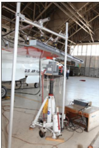
Figure 5. Modal excitation shaker positioned on aircraft structure.
