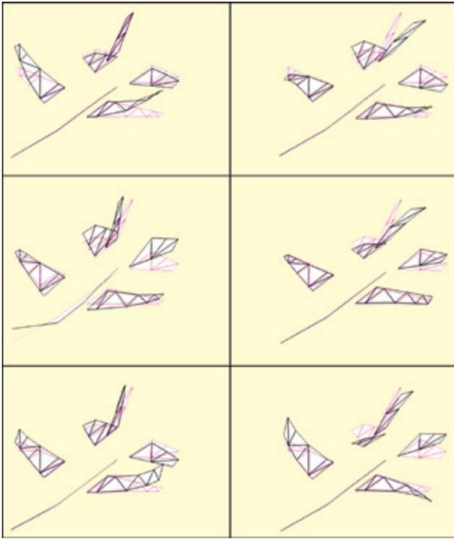
Figure 9. Six mode shapes of the aircraft.
