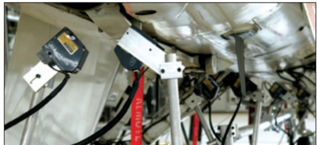
Figure 8. Biaxial DOFs on aircraft belly.
