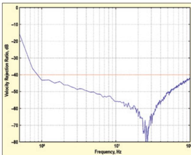
Figure 2. Rejection ratio measurement from typical NIRV sensor.
