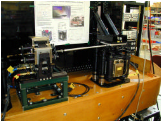
Figure 3. System-level testbed (top). Vertical isolator/actuator and horizontal actuator (bottom left). Hydraulic actuator for shaking platform (lower right).
