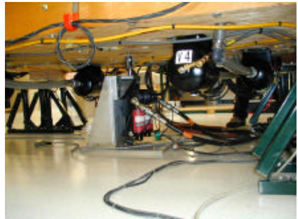
Figure 3. System-level testbed (top). Vertical isolator/actuator and horizontal actuator (bottom left). Hydraulic actuator for shaking platform (lower right).
