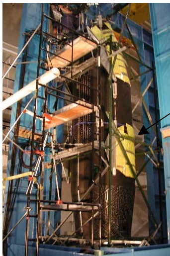
Figure 5. Unistrut LVDT Support Structure
