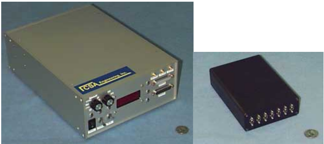
Figure 7: VIS6 electronic support package and load cell signal conditioning support box shown to the same relative scale (US quarter used for reference)
