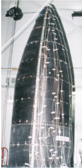
Figure 7. Structural modal testing of STARS fairing
